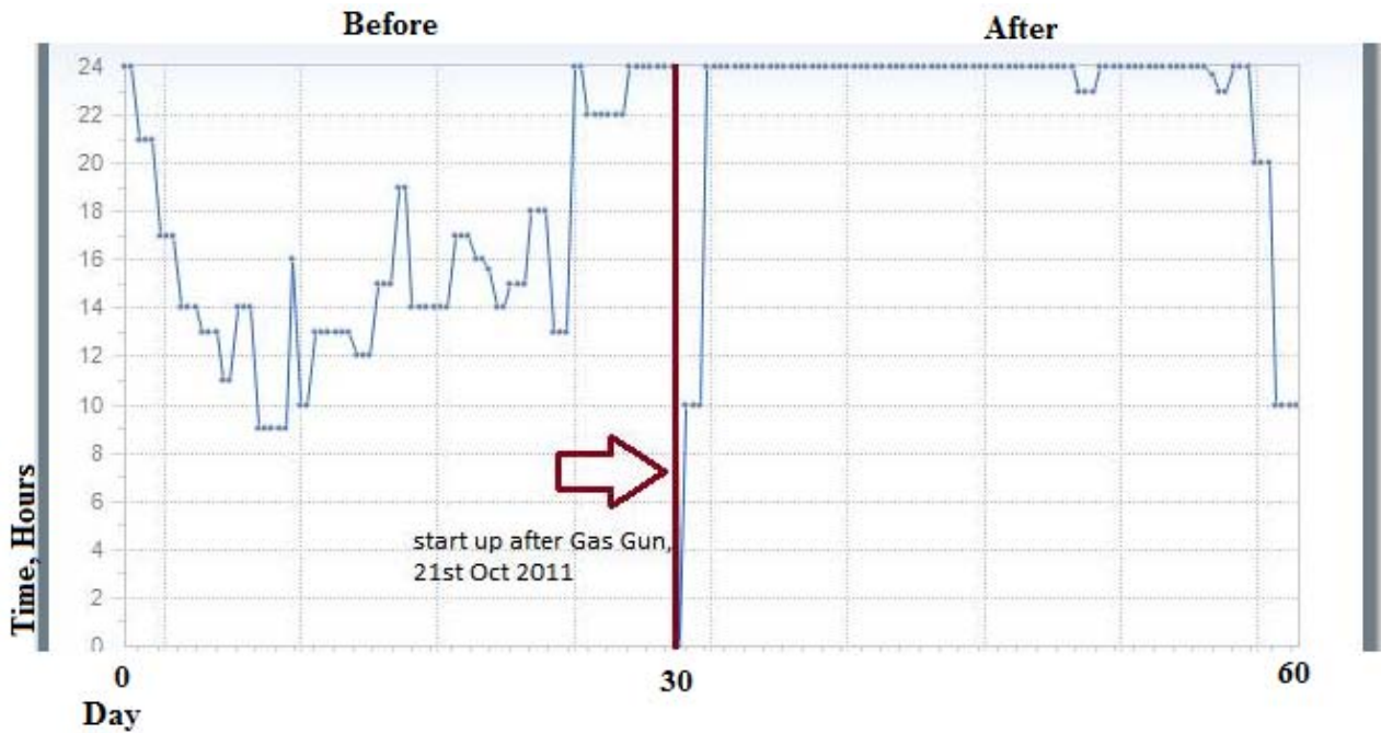
Figure 6 - pump running hours after GasGun treatment
